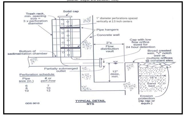
Figure 4-34. Surface Sand Filter Perforated Stand-Pipe (Source: Claytor and Schueler, 1996)
